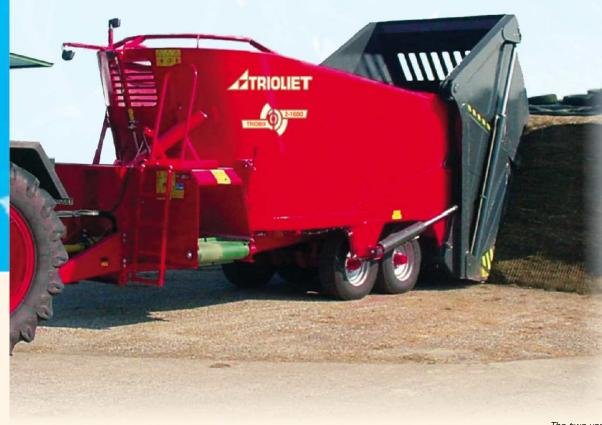
Types Triomix 2 are standard equipped with four single wheels on
