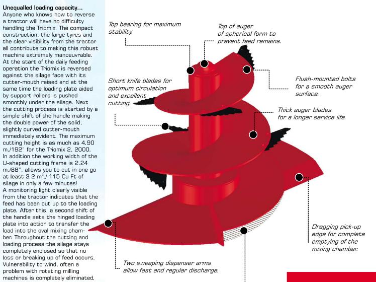
Reduced auger diameter improves vertical circulation and speeds up cutting process.
