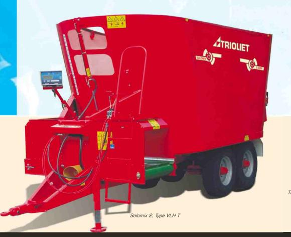
The two vertical mixer augers with cutting blades and planetary gear-drive ensures a perfect TMR result, feed structure
